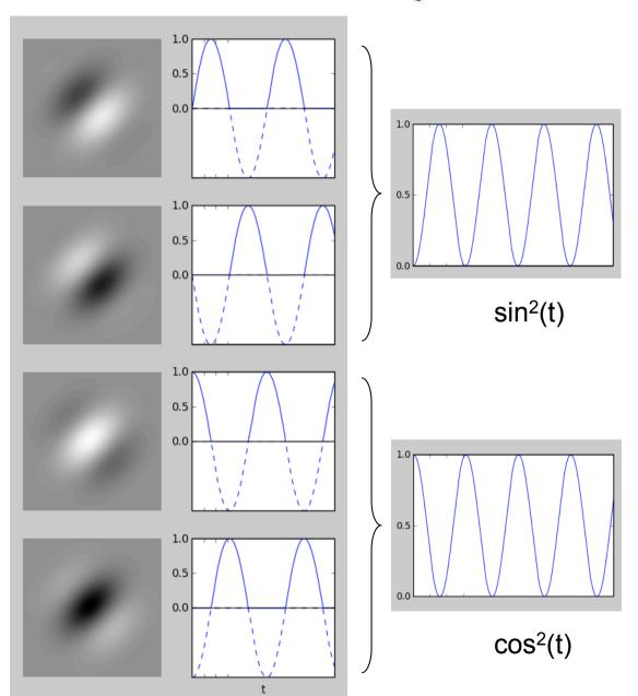
4 model neurons with carrier phases separated by  $\pi/2$
